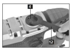
The hammer must be lubricated with grease after approximately 25 hours of operation. Using a cam wrench (12), remove the cover plate (4) from the top of the Machine.
